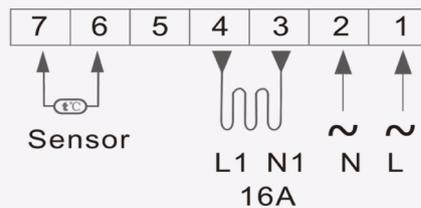
Strip cable to expose 7mm of bare copper and wire up connections as shown:
